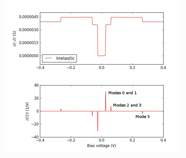
There appear three significant inelastic features (steps in conductance and peaks in IETS). Note that the inelastic conductance is increased by the coupling to the low-frequency transverse modes 0-3 and decreased by the coupling to the high-frequency longitudinal mode 5. Analyzing the scattering states clarifies the reason of the increases.
