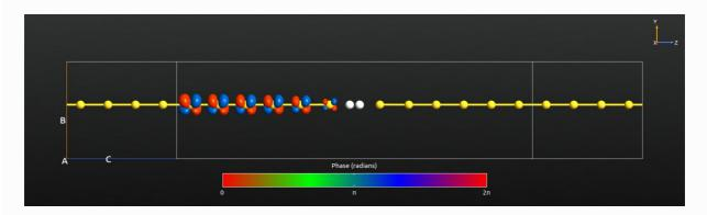
The scattering eigenstate has a clear d-symmetry on the gold chain. Hence, it couples only very weakly to the s-like states of the hydrogen atoms. The elastic transmission is thus small. The coupling to the
